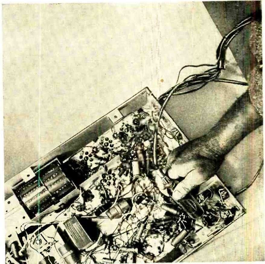
Fig. 7—A low-capacitance probe being used to check the horizontal sync waveforms in the automatic gain control circuit of a television receiver.
