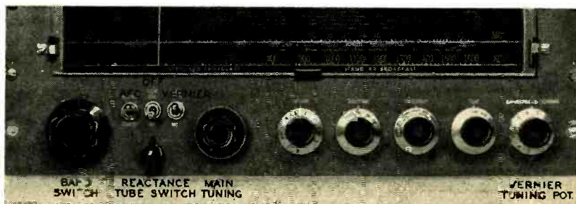
How one vernier control was installed. Spacing from tuning control is wide.
