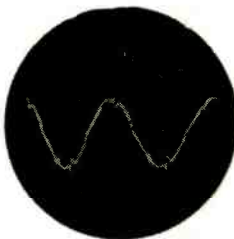
Fig. 10—Scope trace showing considerable r.f. in transmitter power-supply.
