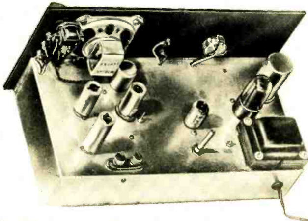
Layout of the signal tracer isolates power supply and high-gain amplifier.
